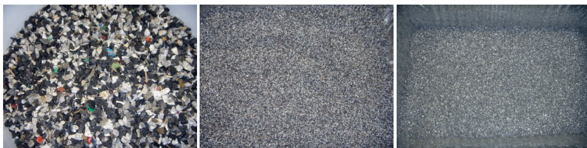
Figuur 13 Monster CIC6 (post shredder residue) – links: origineel, midden: < 1 mm, rechts: < 0.5 mm
