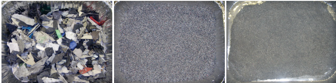
Figuur 16 Monster CIC9 (plastics) – links: origineel, midden: < 1 mm, rechts: < 0.5 mm
