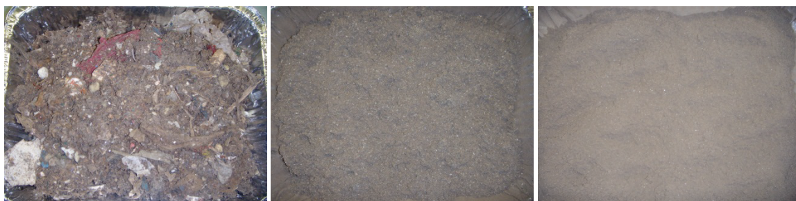
Figuur 14 Monster CIC7 (post shredder residue/fluff) – links: origineel, midden: < 1 mm, rechts: < 0.5 mm
