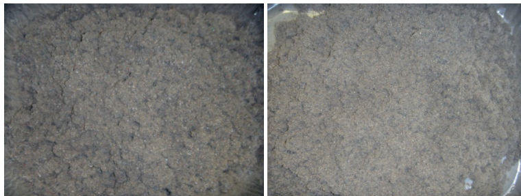
Figuur 9 Monster CIC2 (RDF) – links: < 1 mm, rechts: < 0.5 mm
