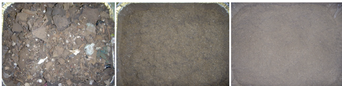
Figuur 12 Monster CIC5 (post shredder residue/RDF) – links: origineel, midden: < 1 mm, rechts: < 0.5 mm
