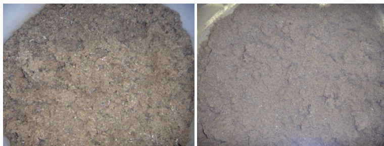
Figuur 10 Monster CIC3 (RDF) – links: < 1 mm, rechts: < 0.5 mm
