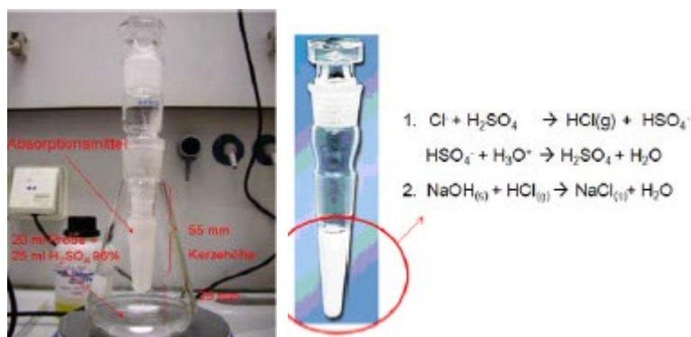
Figuur 10 : NaOH absorber, principe spectroquant COD cell Test, Merck.
