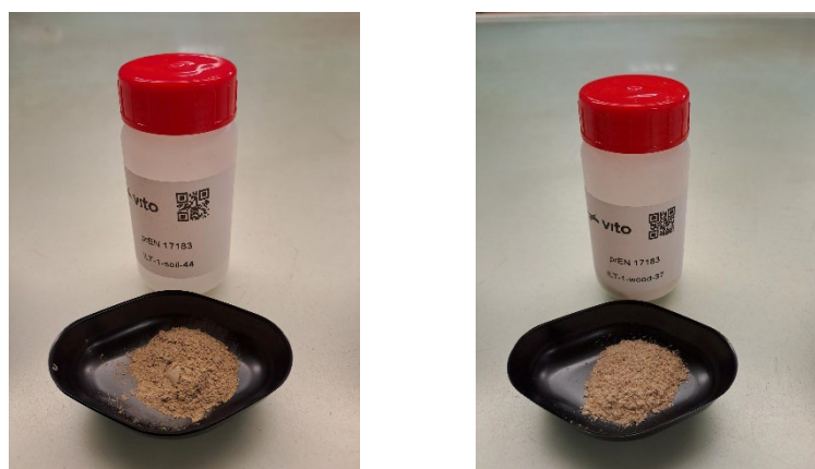
Figure 1 (Left) Soil sample < 250 µm – (Right) Wood sample < 250 µm
