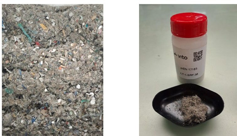
Figure 3 (Left) original SRF – (right) SRF < 500 \mu\text{m} after cryogenic milling
