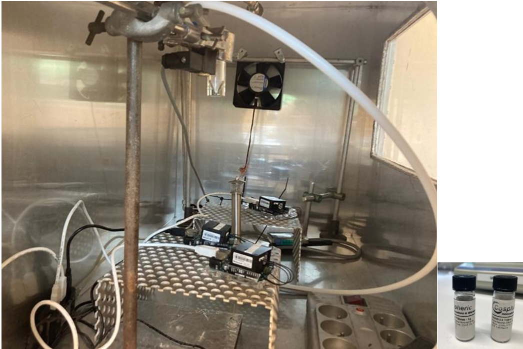
Figure 18: Set-up for PM coarse test (left) and co-spheric dust used for the generation of fine and coarse dust (right)
