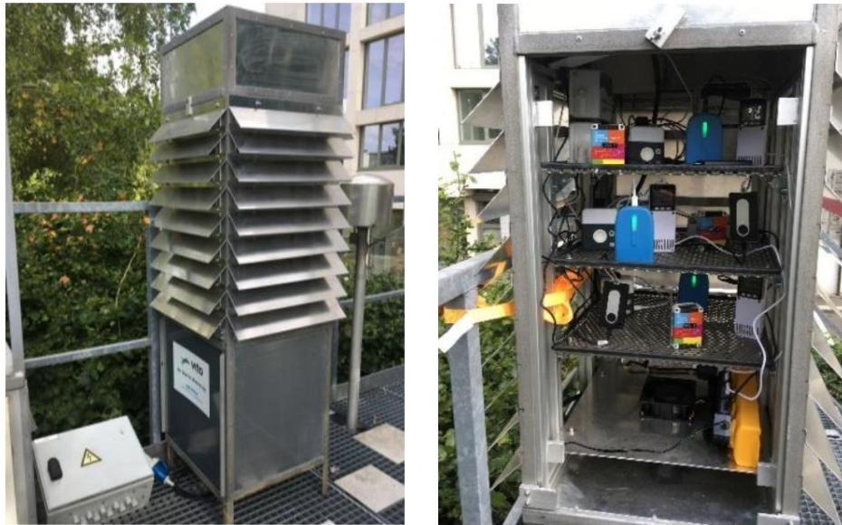
Figure 23: Exposure shelter for sensors (left: outside of the shelter and right: inside with sensors)
