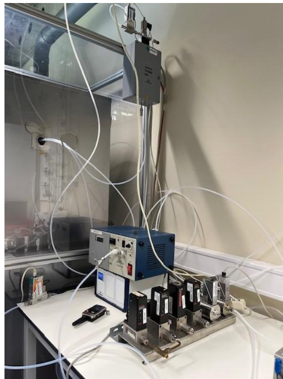
Figure 4: Gas generation system and humidification of inlet air to the test chamber
