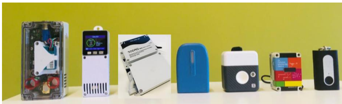
Figure 20: PM sensors tested as part of the benchmark study (from left to right): PAM (2BTech), GeoAir, SODAQ NO2 (SODAQ), SODAQ Air (SODAQ), PMscan (TERA), Open Seneca (Open Seneca) and ATMOTube Pro (ATMO).
