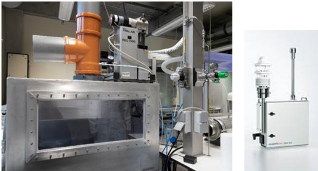
Figure 17: Exposure chamber with generation system on top (left) and reference instrument
