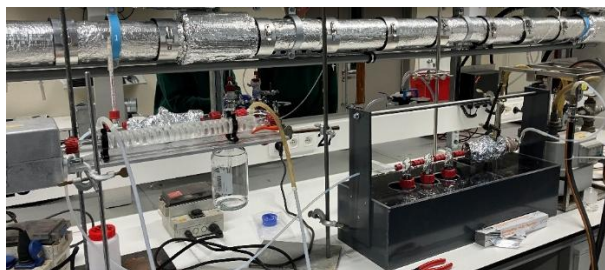
Figure 7 Schematic representation of the “OTM-45 variant” sampling train as described in the LUC/VI/003 compendium procedure (left) and picture of the applied LAB F2 ILC setup (right)
