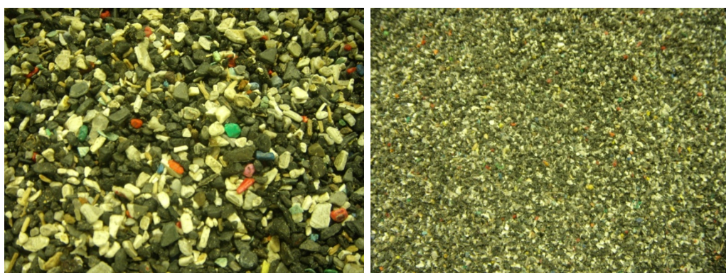
Figuur 15 Monster 13: Shredder granulaten (plastics)(links:origineel; rechts: <1 mm)
