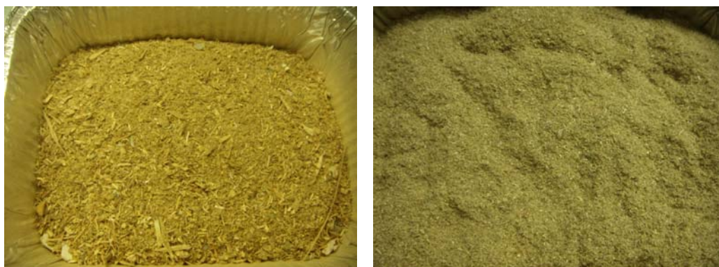
Figuur 3 Monster 1: MDF residu (links: origineel; rechts: < 1 mm)
