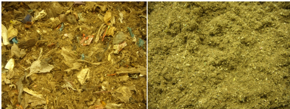
Figuur 11 Monster 9: Fluff RDF (links:origineel; rechts: < 1 mm)
